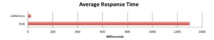
The average response time on disk was 1.3 seconds, with many request taking 30 seconds or more. The Fusion ioMemory based instance showed an average response time of 24 milliseconds, with sub-second responses for every request. Overall, the Fusion ioMemory-based instance showed a 54x improvement in response times over the disk-based system.
